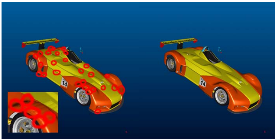
Figure 1. 4 Bits of Subpixel Precision (Left) vs. 12 Bits on the NVIDIA Quadro FX (Right)
